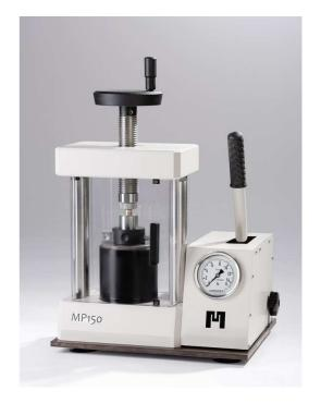
The MP150D can be combined with an adjustable pressure limiter (p/n: MP-S1). With this special feature, you can set the maximum pressure you like to have directly at the display. The pressure will then stop at this point, even if you continue to pump. This saves the die set from overload and makes every press process reproducible.
