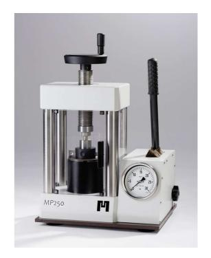
The MP250D can also be combined with an adjustable pressure limiter (p/n: MP-S2) to set the maximum pressure you like to have directly at the display. The pressure will then stop at this point, even if you continue to pump. This makes every press process reproducible. And if different persons are working with this press, they cannot accidentally overload the die set.
