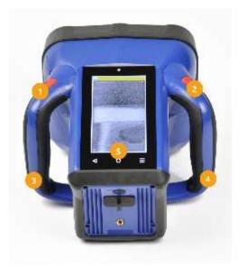
1 & 2 Dual safety triggers to initiate a scan with either hand.
